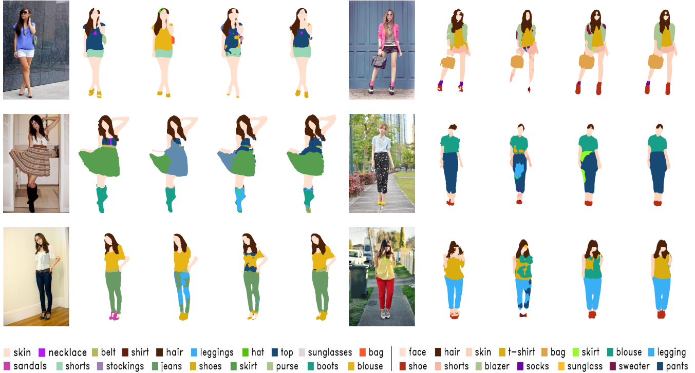
Fig. 3: Left column shows results of the proposed model on Fashionista [2] dataset and right column shows results on CFPD [3] dataset. For each image, first segmentation map denotes the groundtruth annotation followed by results of FCN-8s [5], Outfit Encoder [8] and the proposed model respectively. Notice how the characteristic textures of ‘top’, ‘skirt’, ‘pants’, ‘jeans’ etc. in the images shown help in successfully refining the segments and their corresponding class label predictions.
